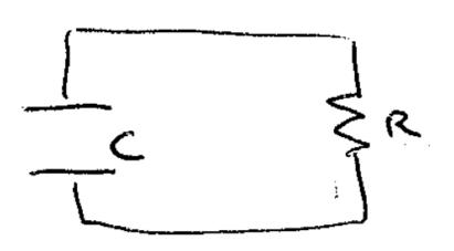
Initially, voltage across the capacitor is 10 volts and it discharges
